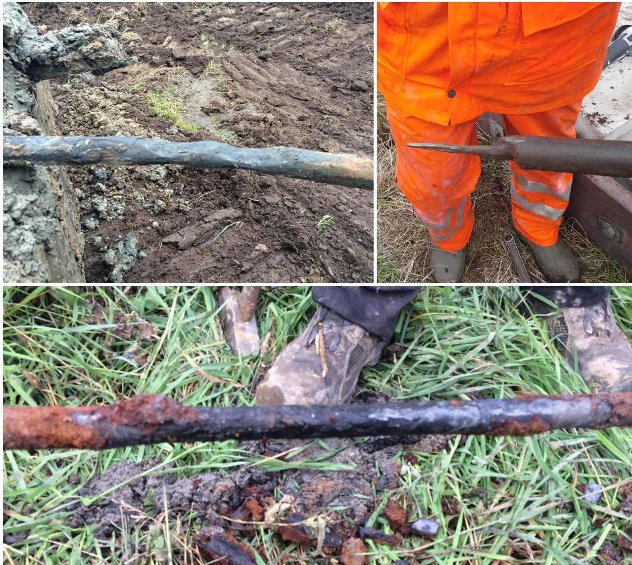
**Figure 4.** Corrosion of steel can be quite severe in areas underlain with acid sulfate soils. Photos: ©Fingrid.
